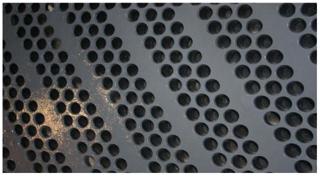
This picture is a cross-section example of Curran's thick film Tube-sheet coating. This is the same coating (different color) as in the case above.
