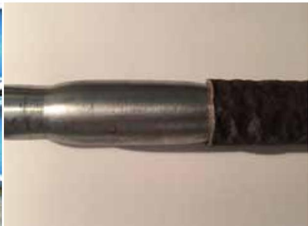
**Stainless steel liner within a carbon steel parent tube**
