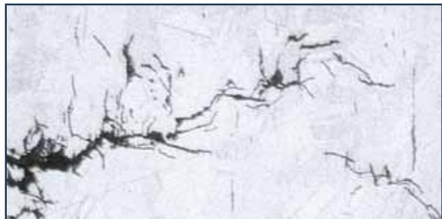
**Fig 2: Highly-branched transgranular cracks penetrating from OD tube wall. Magnification ~100X**
