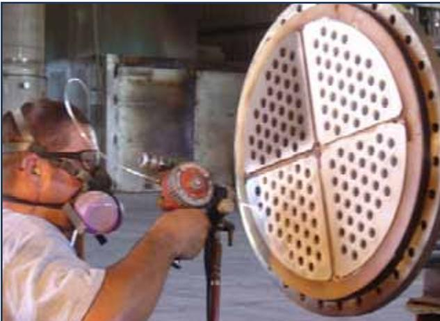
Curran application of “pure silver” using gas acetylene combustion method.
