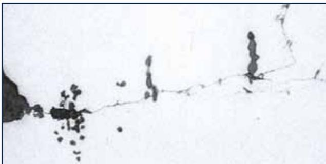
**Fig 1: Cross-section view of tunnel pits and crack tube. Magnification ~200X**
