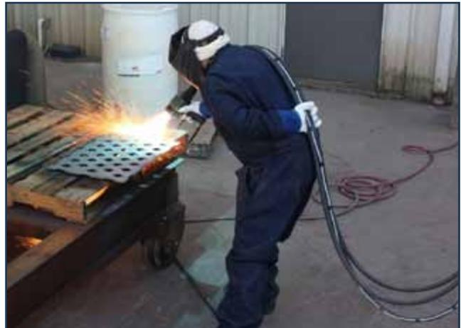
Electric arc facilitates use of broader range of materials, including surface hardening “alloy” to protect mild steel in oxidizing service
