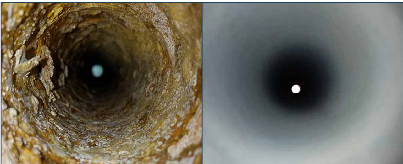
Image of fouled tube ID (L) in sulfur service: risk of under deposit corrosion and impact heat transfer; grit blasted tube (R) facilitates accurate NDE, and returns heat transfer duty. Dry grit does not react with sulfur waste debris, and is highly containable.
