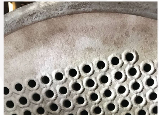
Uncoated tubesheet (top) compared to coated tubesheet; comparable operating period in cooling water.
